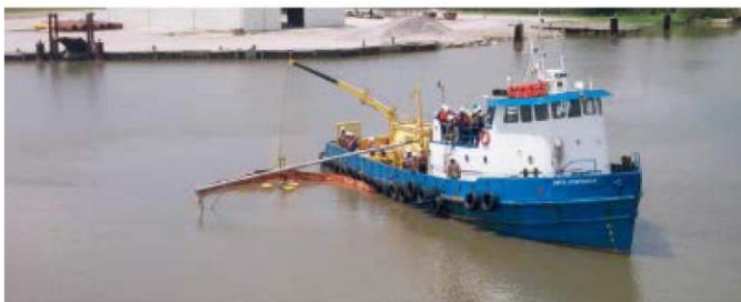
The VOSS (yellow) is being deployed and connected to an out-rigged arm. This is suitable for collection in both large pockets of oil and for recovery of streaming oil.
