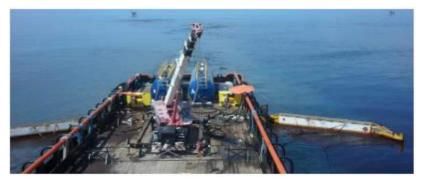
This is a depiction of the same operation as above using KOSEQ Arms. In this configuration, the collecting boom speed dictates the operational pace at  $\leq 3$  knots to minimize entrainment of the oil.
