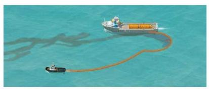
Through the use of an additional VOO, and using extended sea boom, the swath of the VOSS is increased therefore maximizing the oil-to-skimmer encounter rate. Skimming pace is  $\leq 1$  knot.
