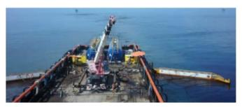
This is a depiction of the same operation as above but using KOSEQ Arms. In this configuration, the collecting boom speed dictates the operational pace at  $\geq 1$  knot to minimize entrainment of the oil.
