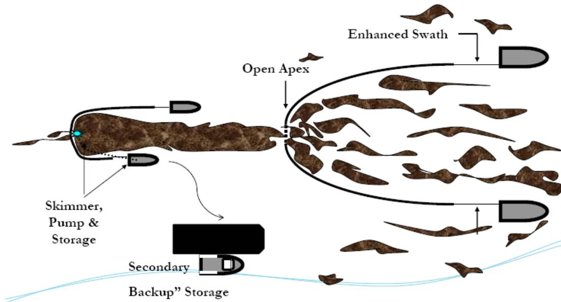
Scattered oil is “caught” by two VOO and collected at the apex of the towed sea boom. The oil moves through a “gate” at that apex, forming a larger stream of oil which moves into the boom of the skimming vessel. Operations are paced at  $>1$ . A recovered oil barge stationed nearby to minimize time taken to offload recovered oil.
