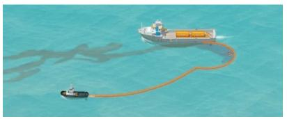
Through the use of an additional VOO, and using extended sea boom, the swath of the VOSS is increased therefore maximizing the oil-to-skimmer encounter rate. Skimming pace is  $\leq 1$  knot.
