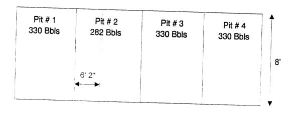
Mud pits #1, #2, #3, & #4 equipped with (1) Brandt Electrical Mud Agitator powered by a 20 Hp motor
