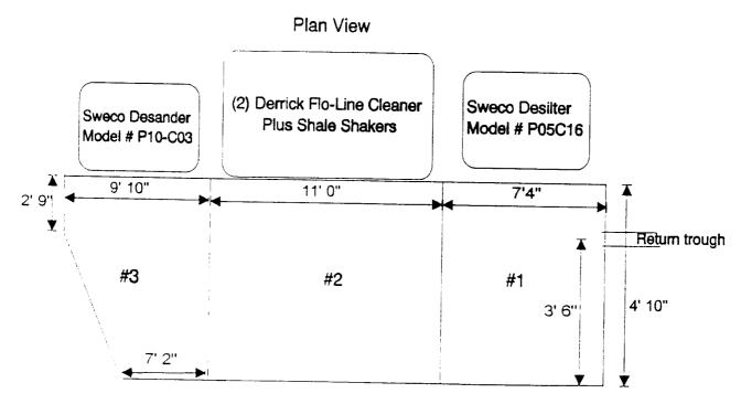
Desander & Desilter discharge into Pit # 1. Desander & Desilter can intake from any pit. Shale Shakers can discharge into any pit.
