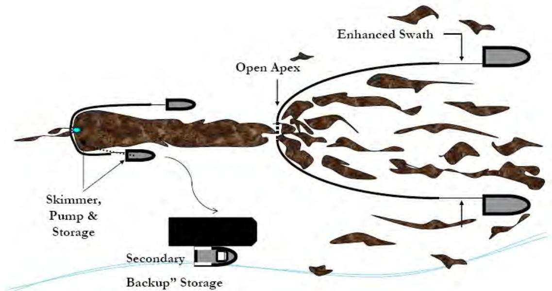
Scattered oil is “caught” by two VOO and collected at the apex of the towed sea boom. The oil moves through a “gate” at that apex, forming a larger stream of oil which moves into the boom of the skimming vessel. Operations are paced at  $>1$ . A recovered oil barge stationed nearby to minimize time taken to offload recovered oil.
