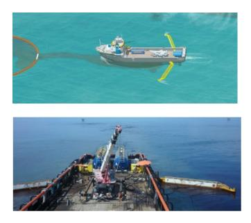
This is a depiction of the same operation as above but using KOSEQ Arms. In this configuration, the collecting boom speed dictates the operational pace at  $\geq 1$  knot to minimize entrainment of the oil.
