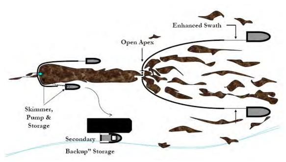
Scattered oil is "caught" by two VOO and collected at the apex of the towed sea boom. The oil moves thought a "gate" at that apex, forming a larger stream of oil which moves into the boom of the skimming vessel. Operations are paced at >1. A recovered oil barge stationed nearby to minimize time taken to offload recovered oil.
