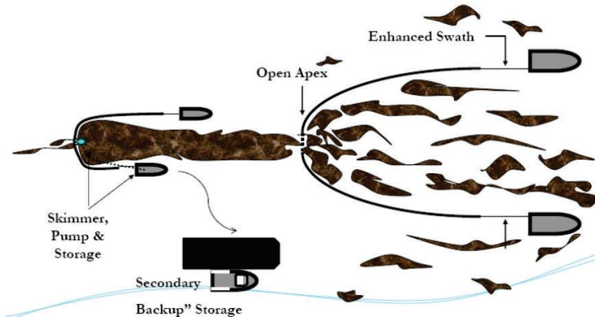
Scattered oil is “caught” by two VOO and collected at the apex of the towed sea boom. The oil moves thought a “gate” at that apex, forming a larger stream of oil which moves into the boom of the skimming vessel. Operations are paced at >1. A recovered oil barge stationed nearby to minimize time taken to offload recovered oil.
