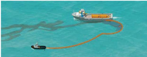
Through the use of an additional VOO, and using extended sea boom, the swath of the VOSS is increased therefore maximizing the oil-to-skimmer encounter rate. Skimming pace is  $\leq 1$  knot.
